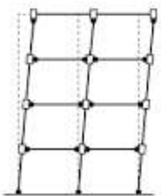
Failures in beams Buildings could keep standing
