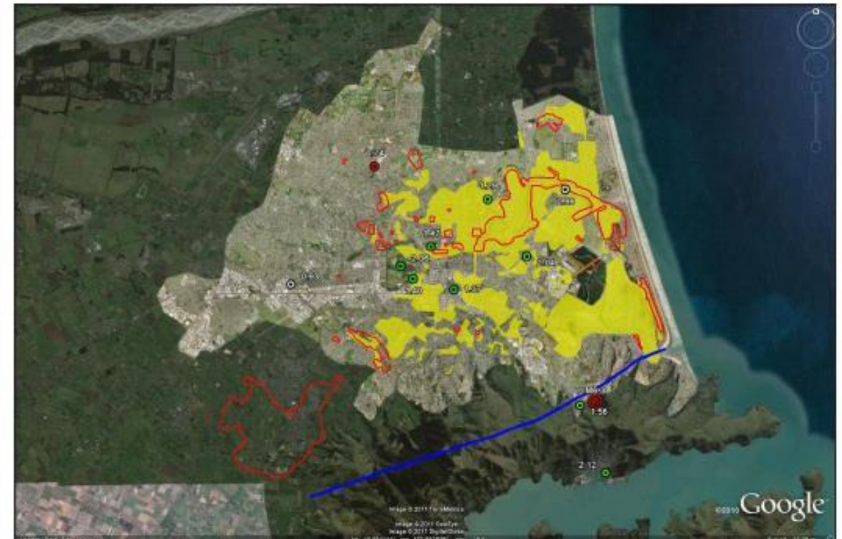
Figure 3. Liquefaction in February 2011 (green) and September 2010 (red contours) (courtesy of R. Green; GEER 2011).
