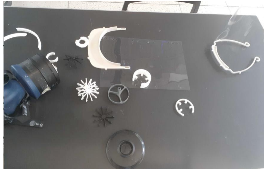
3D Printed Components of Face Shield developed in Australia
